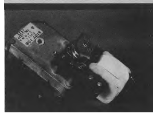
(Above) A small transformer with its frame removed. The arrow points to a loosened lamination. (Right) A synchronous induction motor. Eddy currents induced in the armature eliminate the need for expensive and noisy commutators. Motors like these are cheap and reliable but very inefficient.
