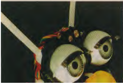
This Furby's head, stripped of its outer covering and fur; reveals the light sensor between the eyes. On either side are infrared transmitter and receiver LEDs. Furbys can automatically communicate with one another via this infrared link.
