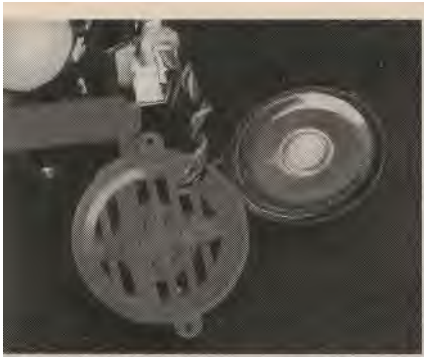
The Furby's 2-inch speaker is capable of very clear sound reproduction.
