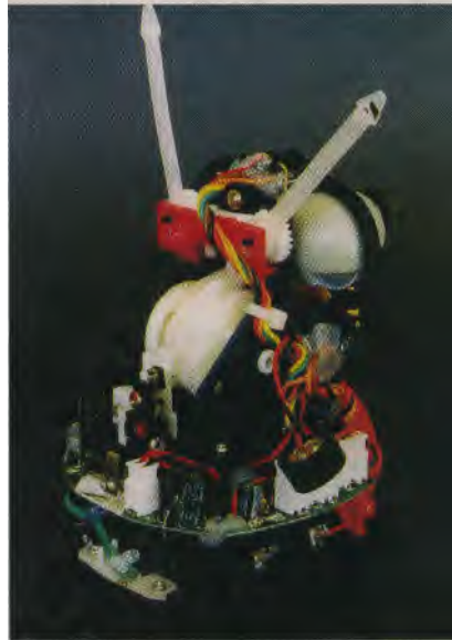
This photo shows just how jam-packed a Furby is inside. A semicircular PC board is located just above the battery compartment, with the mechanical module mounted on top of that. The sound-sensing microphone is hanging on its lead in the foreground.
